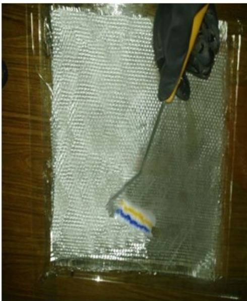
Figure (5): Manufacture of (F/P comp.) material using hand lay-up method
