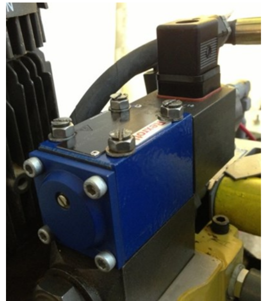
Figure (3) Proportional pressure relief valve type DBEP 6 A06-13/45AG24K4M
