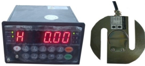
Plate (7) Load Cell and Digital Indicator
